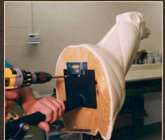
Permanently secured by screws through stand and into form backboard.
