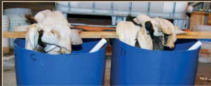
Static rehydration and separate pickle bath in a plastic container.
