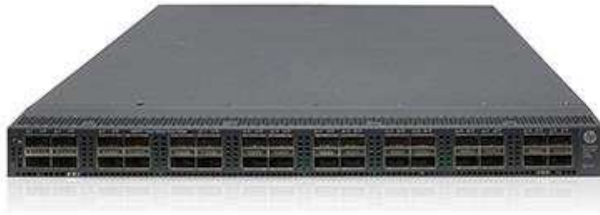
Figure 13. HP 5930-32QSFP+ 40GbE Aggregation switch
