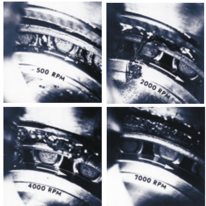
Pumping effect of a tapered roller bearing
