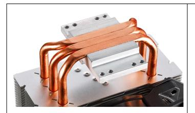
By compressing heatpipes together there is 45% more surface area on the cooler base which improves heat dissipation compared to previous version (CDC 1.0)
