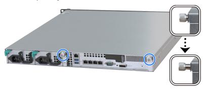
**b** Remove the top cover by firmly grasping the thumb grooves and pulling in the direction indicated below, and put the top cover aside.
