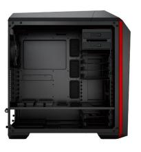
**Dual chamber design** – Partition plate isolates power supply and give options for clean cable management.
