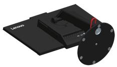
Step 3: Remove the base and stand from the monitor.
