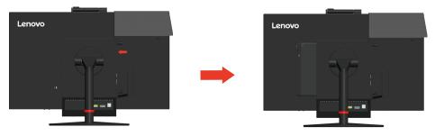
3. Pull the computer out of the computer bay. Then, pivot the cable cover as shown to the closed position.
