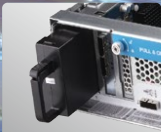
NVRAM Write Cache Protected by Battery
