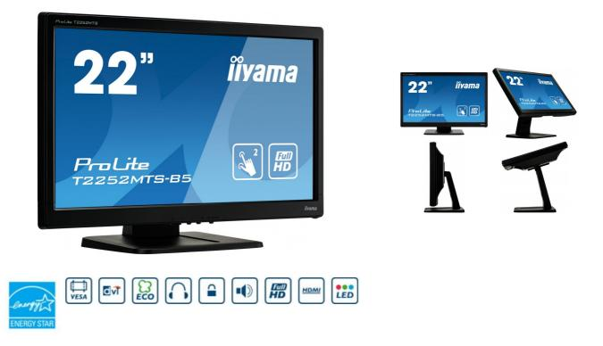
22" Dual Touch screen, based on Optical Touch Screen Technology
