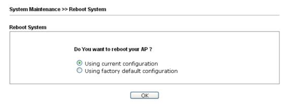
If you want to reboot the modem using the current configuration, check **Using current configuration** and click **OK**. To reset the modem settings to default values, check **Using factory default configuration** and click **OK**. The modem will take 5 seconds to reboot the system.
