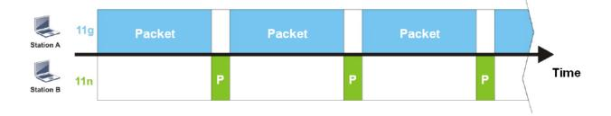
To improve this problem, Airtime Fairness is added for VigorAP 900. Airtime Fairness function tries to assign *similar airtime* to each station (A/B) by controlling TX traffic. In the following figure, Station B(11n) has higher probability to send data packets than Station A(11g). By this way, Station B(fast rate) gets fair airtime and it's speed is not limited by Station A(slow rate).
