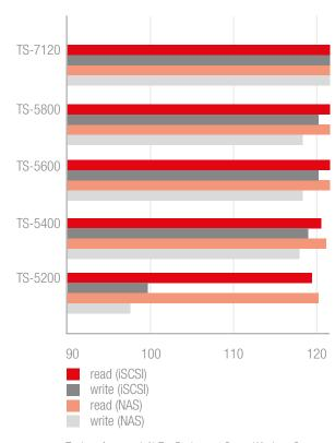
**Test environment:** N-Tec Rackmount Server Windows Server 2008R2, Dual XEON 32 GB RAM, 2 x IntelPRO/1000Dual = 4 x Gigabit NIC; Cisco SG300-10P 10 Port managed Gigabit with PoE.
