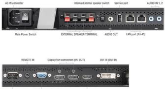
RS-232C (D-Sub 9 pin) VGA IN (mini D-Sub 15 pin)
