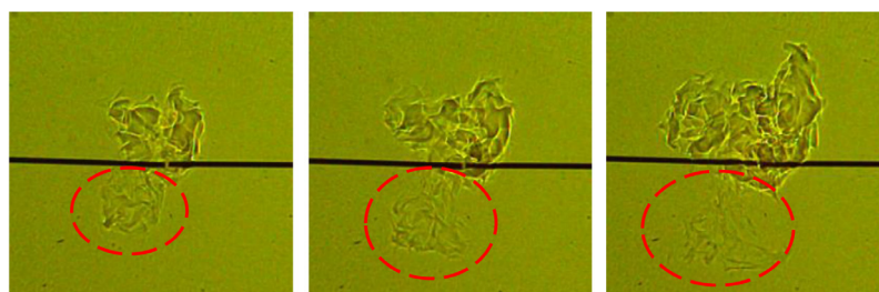
(b) Local extinction at X_{NH_3} = 0.6 , u' = 2.72 m/s and P = 1 bar. The time interval of image is
