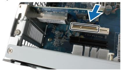
**Note:** Make sure the connector is fully inserted. Otherwise, the network interface card might not be able to function properly.
