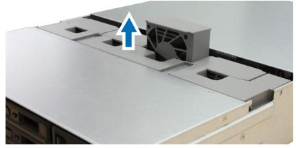
**5** Prepare a new fan, and slide it into the RackStation. Make sure the fan is aligned properly as illustrated below.
