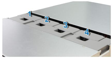
4 Find the malfunctioning fan. Lift the fan upward to remove it.
