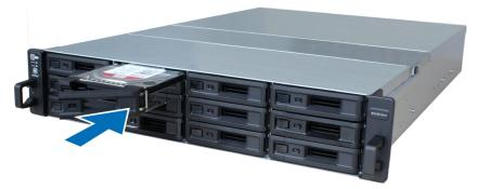
Note: Make sure the tray is pushed in all the way. Otherwise, the drive might not be able to function properly.
