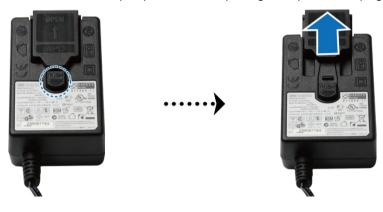
2 Slide the plug adapter provided into the slots by pushing it downward. Note that the plug adapter that comes with your EDS14 varies depending on your region. The image below is for reference only.
