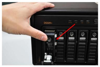
Reminder: Make sure the tray is completely attached to the system. Otherwise, the hard disk might not be able to function properly.
