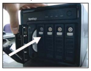
Reminder: Make sure the tray is completely attached to the system. Otherwise, the hard disk might not be able to function properly.
