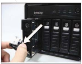
3. Attach the SATA hard disk to the hard disk tray and use 4 screws to fix the hard disk.
