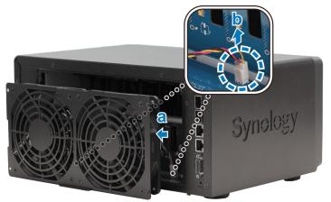
c Remove the 4 screws that secure the malfunctioning fan, and then remove the fan.
