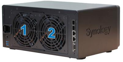
3 Remove the 4 screws that secure the fan panel.
