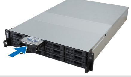
Note: Make sure the tray is pushed in all the way. Otherwise, the drive might not be able to function properly.
