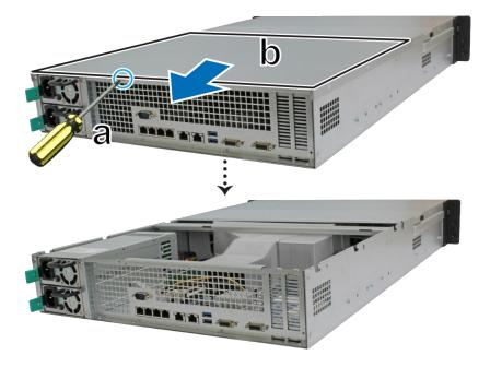
a Remove the screw on the back of RackStation.
