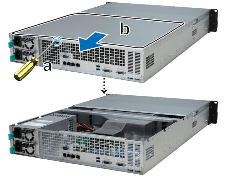
a Remove the screw on the back of RackStation.
