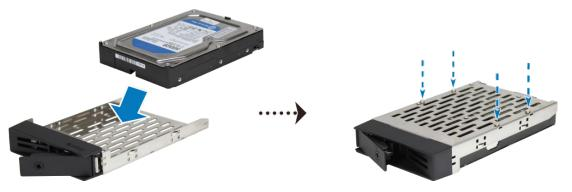
• For 2.5" drives: Place the drive in the drive tray. Turn the tray upside down and tighten screws in the four spots indicated below to secure the drive.
