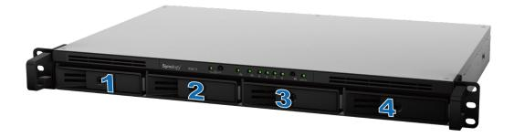
**Note:** If you want to create a RAID volume, we recommend all installed drives be the same size in order to optimize drive capacity usage.
