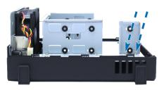
**b** Slide the drive into the hard drive bay, and push it all the way until it's firmly connected to the SATA connector. Secure the drive with the screws provided.
