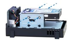
• For 3.5" drives with 2 screw holes on each side (indicated below):
