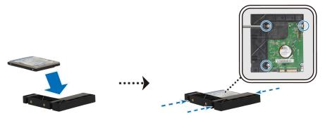
**b** Slide the 2.5" Disk Holder into the hard drive bay, and push it all the way until the drive is firmly connected to the SATA connector. Secure the Disk Holder with the provided screws.
