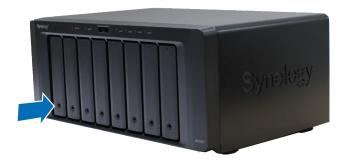
2 Pull the hard drive tray handle in the direction as indicated below to remove the hard drive tray.
