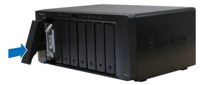
Note: Make sure the tray is pushed in all the way. Otherwise, the drive might not be able to function properly.
