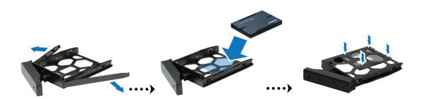
4 Insert the loaded hard drive tray into the empty hard drive bay.
