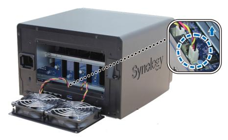
$\boldsymbol{c}\,$  Remove the 4 screws that secure the malfunctioning fan, and then remove the fan.
