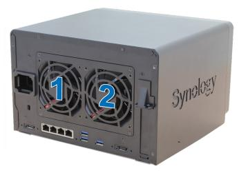
3 Remove the 4 screws that secure the fan panel.
