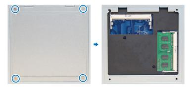
*Important:* When you remove the lid, you expose sensitive internal components. Avoid touching anything other than the memory assembly when you remove or add memory.
