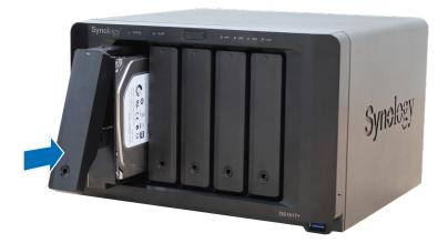
Note: Make sure the tray is pushed in all the way. Otherwise, the drive might not be able to function properly.
