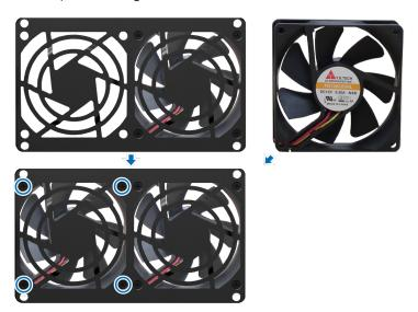
**b** Connect the 2 fan cables to the connectors located near the bottom of the fan socket, and then replace the fan panel.
