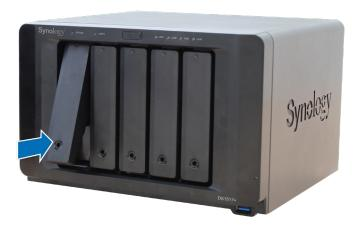
2 Pull the hard drive tray handle in the direction as indicated below to remove the hard drive tray.
