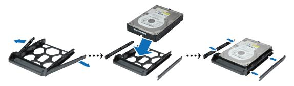
• For 2.5" drives: Remove the fastening panels from the sides of the drive tray and store them in a safe place. Place the drive in the blue area (shown below) of the drive tray. Turn the tray upside down and tighten the screws to secure the drive in place.
