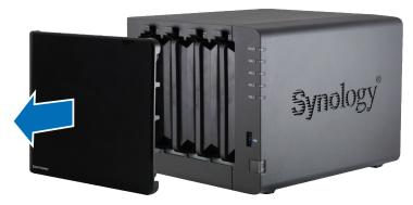
2 Push the latch upward and pull the handle to remove the drive tray.
