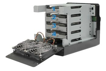
• For 3.5" drives only: It is recommended that you secure the drive trays with the screws (for securing drive trays) provided. For drives without the central mounting holes, you can skip this step.
