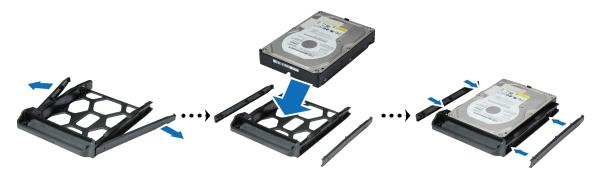
• For 2.5" drives: Remove the fastening panels from the sides of the drive tray and put them in a safe place. Place the drive in the blue area (shown below) of the drive tray, turn the tray upside down, and then tighten the screws provided to secure the drive.
