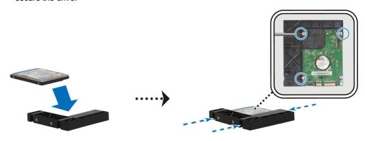
**b** Slide the 2.5" Disk Holder into the hard drive bay, and push it all the way until the drive is firmly connected to the SATA connector. Secure the Disk Holder with the provided screws.
