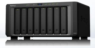
Synology DiskStation DS1817 is the first value series model featuring two built-in 10GBASE-T ports and upgradable RAM module, and is powered by quad-core processor with hardware encryption engine and expandable scalability of up to 18 drives. DS1817 is the ideal solution for centralizing data backups, protecting critical assets, and sharing files across different platforms. Synology DS1817 is backed by Synology's 3-year limited warranty.
