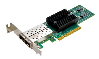
Synology E10G17-F2 is a dual-port 10 Gigabit SFP+ PCle 3.0 x8 Ethernet adapter specifically designed for Synology XS+/XS series NAS servers. With CPU Offload (RDMA over Ethernet)<sup>1</sup> support, E10G17-F2 satisfies the demands on high performance computing. Synology E10G17-F2 is backed with Synology's 5-year limited warranty.
