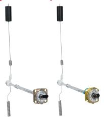
Here is an adjustable, magnetic, liquid-level gauge which makes it a snap to quickly and economically replace non-functional LP Gas gauges in the field. Because one size adjustable gauges fit many tanks, the 'One' Gauge greatly reduces the number of spare gauges you need to stock. The 'One' Gauge is UL listed for LP gas service.
