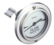
Indicates direction of flow of compatible liquids in pipe lines at working pressures up to 600 psig up to 160°F. The indicator must be installed in pipe line tees. Specify Part Number and "A" Dimension
