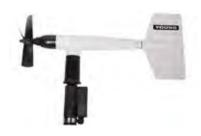
The FTS SDI RMYoung Wind Monitor is the RM Young 05103 wind monitor with the addition of an SDI-12 interface. It's the only mechanical dual wind sensor available that offers SDI output. The SDI-12 interface avoids the complexity of measuring the AC wind speed signal or the potentiometer output. Wind speed and wind direction are returned in engineering units when requested by SDI command.
