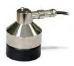
The SDI-SR50A is a rugged acoustic sensor for measuring the distance from the sensor to a target. It is typically used to measure snow depth. It uses a multiple echo processing algorithm to help ensure measurement reliability.
