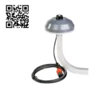
The SDI-PYR is a pyranometer that measures total light available (global sun plus sky radiation). The sensor converts light through a photodiode to an electrical signal which is interpreted by the internal microprocessor.
