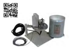
The RG-E12-30 heated rain gauge is a high precision tipping bucket. Approved to CSA (Canadian Standards Association) special inspection standards and meeting U.S. Field evaluation requirements, the RG-E12-30 offers exceptional calibration retention.
