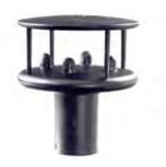
Ultrasonic wind speed and direction sensors offer an alternative to conventional cup and vane or propeller type wind sensors. They are robust and lightweight with no moving parts, and use an SDI-12 interface, therefore offering several advantages over analog sensors. This sensor is suitable for land or marine applications.
