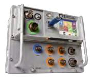
The Axiom H2 is a rugged datalogger (DCP) designed for remote data collection and complex SDI-12 sensor applications. It features four independent, electrically isolated SDI-12 ports that can each handle up to 500mA, and an integrated solar regulator.
