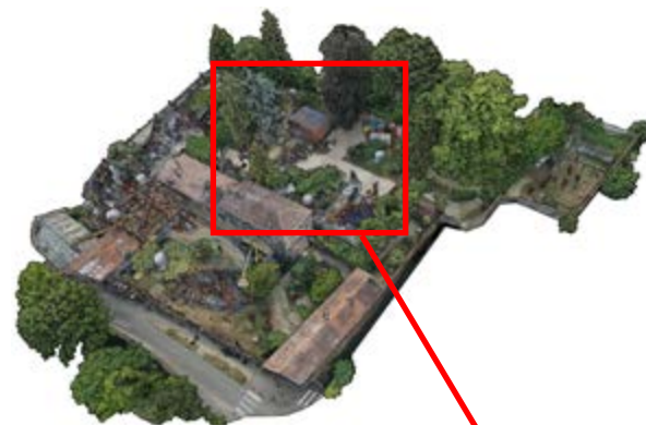
Images made from point clouds: different levels of scale and interpretation. Resolution: 1 pixel : 1 cm colored (TTGE survey, 2020)
