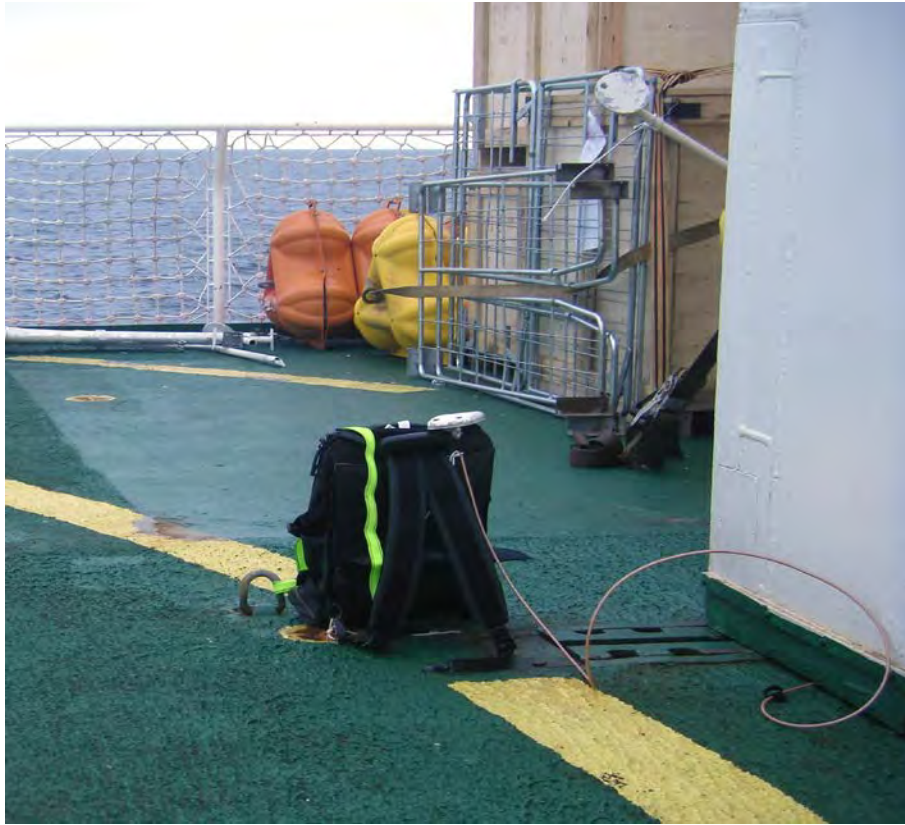
Figure 5.7. GPS antenna for the GT-1A while the helicopter was hangered. The rigid framed backpack strapped to the helo deck proved to be adequate as an antenna mount and sufficiently nonintrusive to other deck operations.
