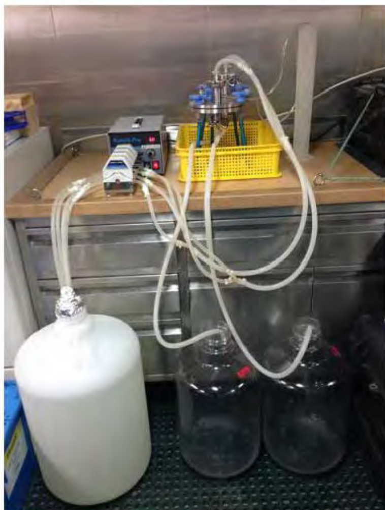
Figure 3.14. Photos of a large volume seawater filtration system used in the present study.
