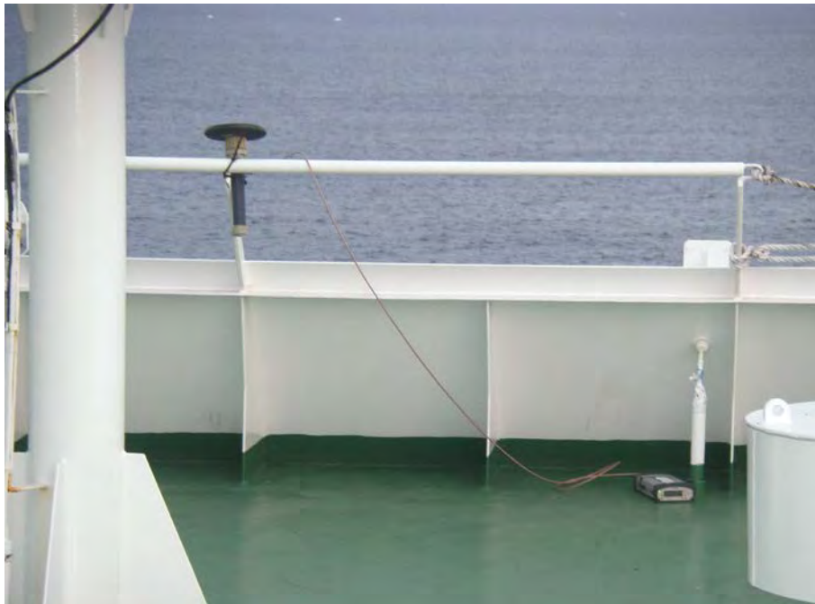
Figure 5.8. Base station GPS receiver and antenna installed on Compass Deck of RV Araon during gravity data acquisition flights.
