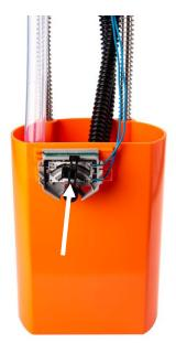
**STEP 10:** Install the SureFlo assembly into the tank, use caution with the float arm and do not over-rotate the pump once installed.
