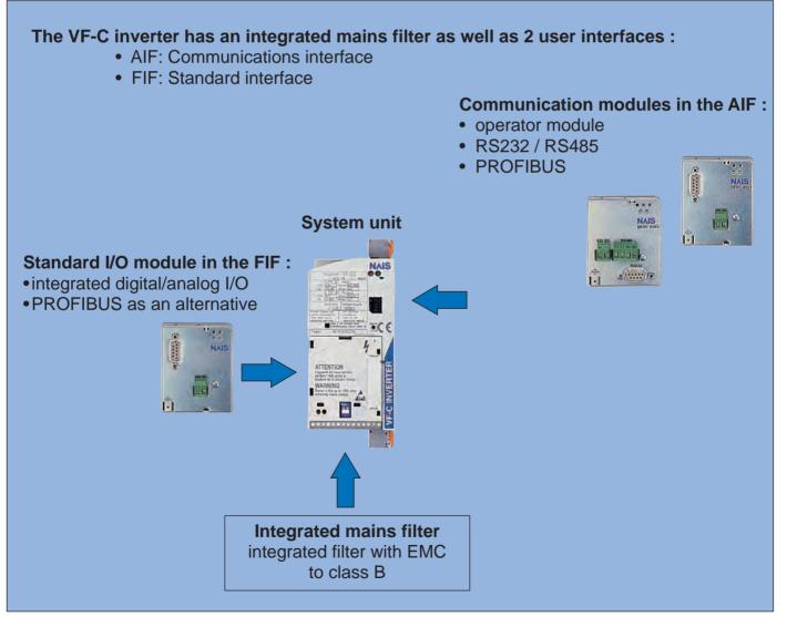
The standard I/O module (order number: BFVC90XY) is included in the VF-C inverter. It need not to be ordered separately.
