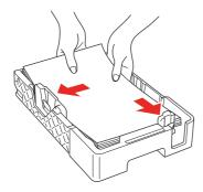
Squeeze the edge guides and slide them against the paper. Make sure the paper is stacked against the front edge guide.
