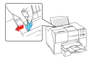
Insert paper with the printable side up, against the right side of the feeder. Then slide the edge guide against the paper.
