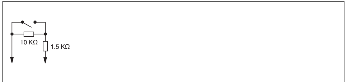
Figure 6.85 Mechanical contact with additional resistor circuit
