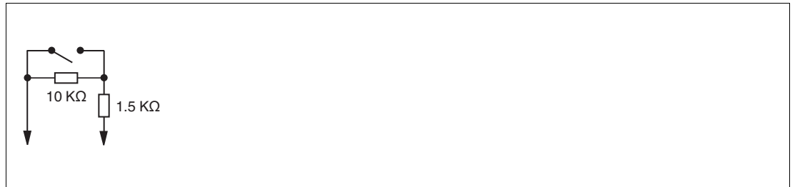
Figure 6.13 Mechanical contact with additional resistor circuit
