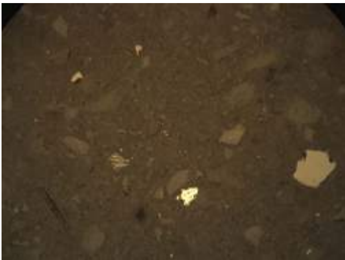
P3S Bulk Tailings: A) Cross Polarized Light, Field of View = ~0.8 mm, B) Plain Polarized Light, Field of View = ~0.8 mm, C) Reflected Light, Field of View = ~0.8 mm
