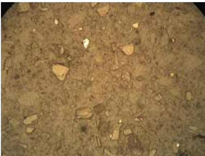
P1S Bulk Tailings: A) Cross Polarized Light, Field of View = ~0.8 mm, B) Plain Polarized Light, Field of View = ~0.8 mm, C) Reflected Light, Field of View = ~0.8 mm
