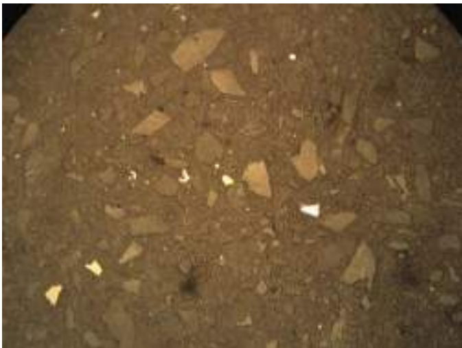
P2S Bulk Tailings: A) Cross Polarized Light, Field of View = ~0.8 mm, B) Plain Polarized Light, Field of View = ~0.8 mm, C) Reflected Light, Field of View = ~0.8 mm
