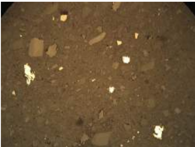
P1Solids Bulk Tailings: A) Cross Polarized Light, Field of View = ~0.8 mm, B) Plain Polarized Light, Field of View = ~0.8 mm, C) Reflected Light, Field of View = ~0.8 mm
