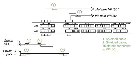
When connecting the Ethernet cable, the VP1801 automatically detects TX/RX , plus and minus connections, and switches to the correct connection.
