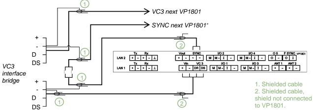
\* The SYNC connection is necessary for HDX ISO synchronization between other readers. For FDX a SYNC connection is possible, but not necessary if only one antenna is used. When two antennas are used the SYNC connection is always needed, even when FDX-only (no ISO) mode is enabled. The switching between the two antennas uses the ISO timing.
