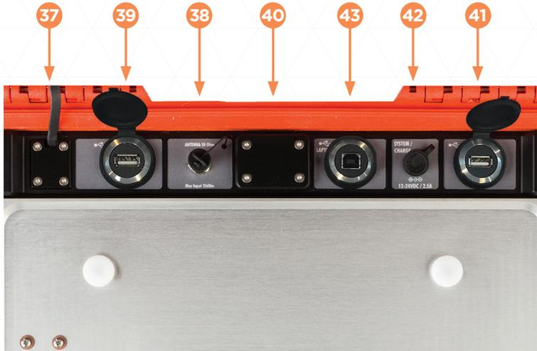
Figure 8: Input/Output Panel
