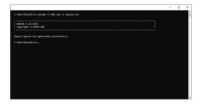
AMISDE is a command line tool for exporting setup data from an Aptio® ROM image. It produces a helpful summary report of BIOS parameters and default values that enhances productivity in testing and manufacturing.
