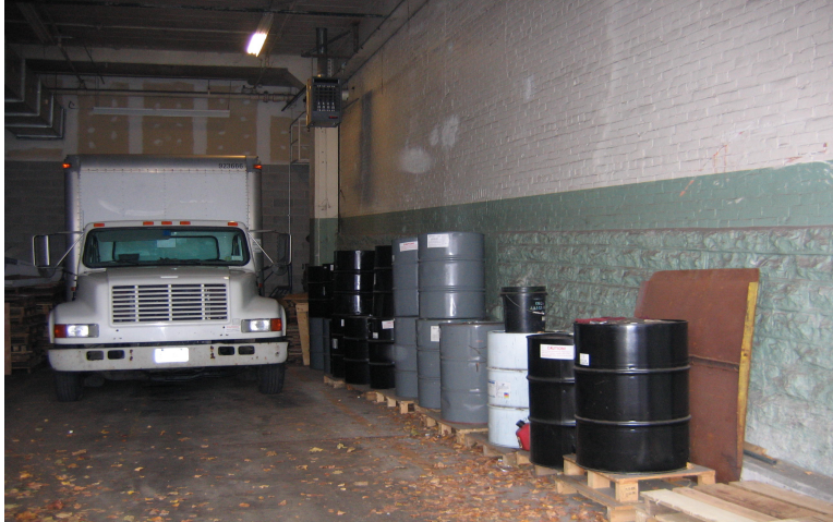
Photo 10: View of the 55-gallon drums used to store waste solvents. The drums are picked up by Safety Kleen on an as needed basis. Drums should be on a drum containment/spill platform.
