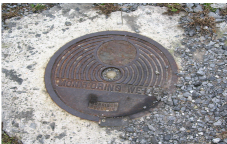
Photo 6: View of the monitoring well potentially associated with the 30,000-gallon UST that was formerly located in the vacant lot behind Century Centre I.
