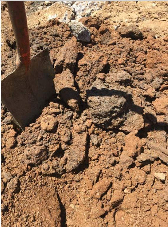
Photo 15: Discrete soil contamination consisting of gray fine to medium sand, trace silt, damp with a petroleum odor. Photo taken June 20, 2017.
