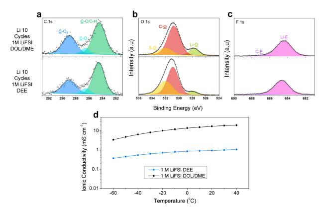
**Figure 3.**Lithium SEI and ionic conductivity study of electrolytes. Ex-situ XPS of Li anodes after 10 cycles for 1 mAh cm<sup>-2</sup> at 0.5 mA cm<sup>-2</sup> in 1 M LiFSI DOL/DME and 1 M LiFSI DEE at room temperature. **a)** C 1s, **b)** O 1s, and **c)** F 1s spectra with assigned peaks from Gaussian/Lorentzian product peak fitting. **d)** Measured ionic conductivity of the investigated electrolytes at different temperatures.
