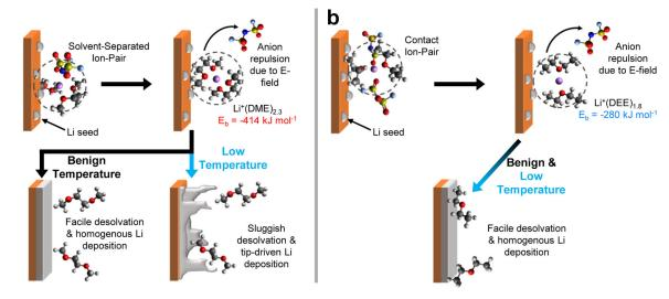
**Figure 5.**Proposed relationship between electrolyte structure and desolvation. Proposed desolvation mechanisms and corresponding Li<sup>+</sup>/solvent binding energies obtained from quantum chemistry simulations in **a**) 1 M LiFSI DOL/DME, and **b**) 1 M LiFSI DEE.
