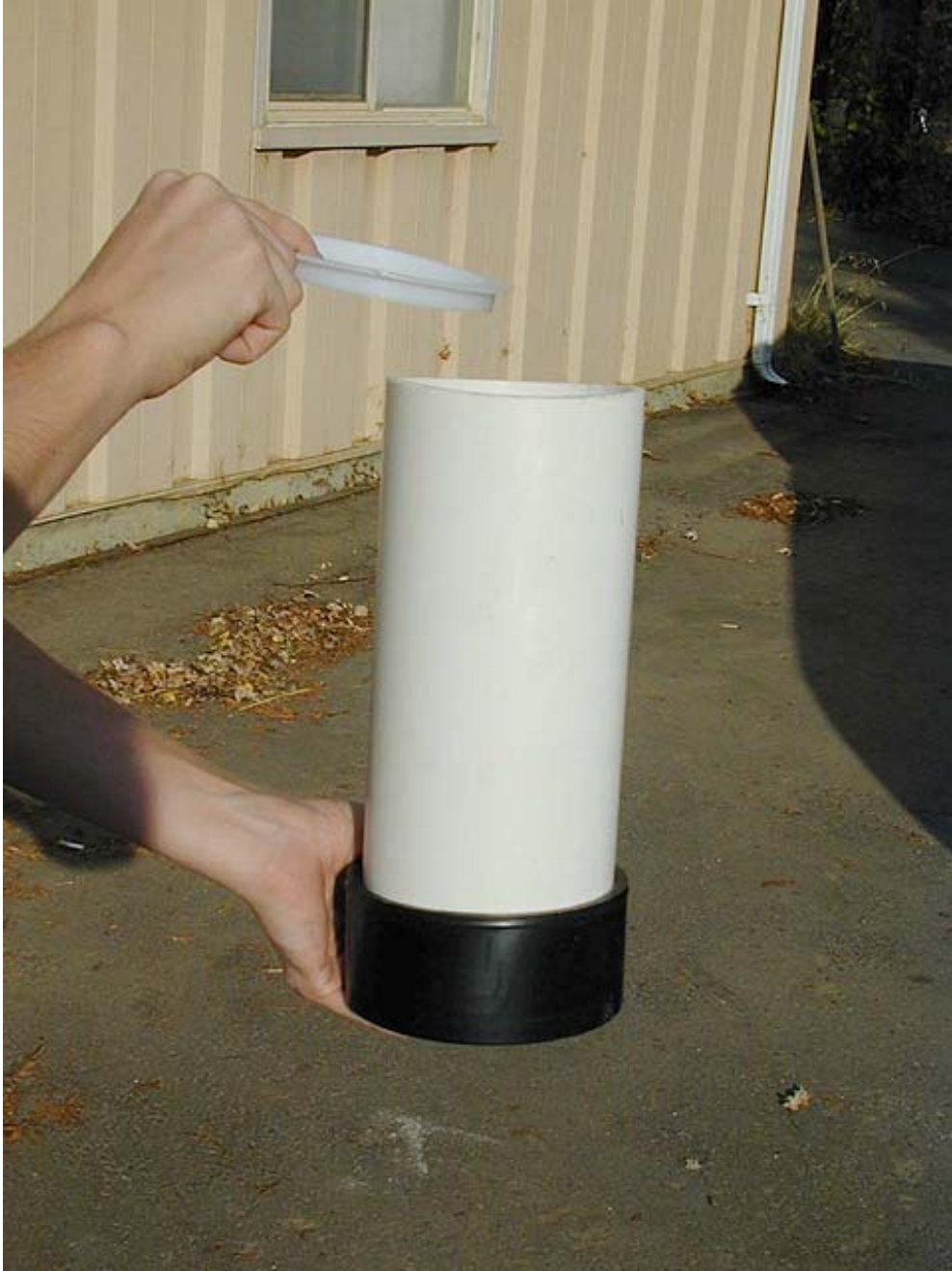
Figure 3. PVC core sampler used for removal and transport of sediment from C. taxifolia infested sites after treatment with chlorine.
