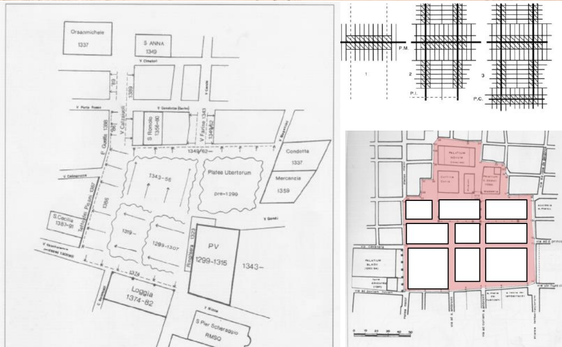
Fig. 1. A project merging two row-houses into one in-line house, Archivio Capitolino di Roma, titolo Fig. 2. Aggregation of row houses on matrix route (1), planned construction route (2), spontaneous connection route (3 above), planned connection route (3 below), (Strappa, 1995). Fig. 3. Reconstruction of the Curia Communis Bononiae, at the time of the terminatio of 1294, in red the blocks that were demolished (Guidoni & Zolla 2000). Fig. 4. The different phases of the definition of Piazza della Signoria in Florence by demolishing urban blocks, (Guidoni, 2002).
