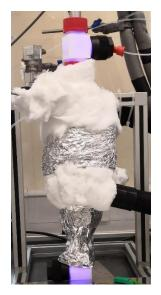
Figure 2.15. Photo of the HPR during low-temperature testing with the PhotoLED in situ. There was a need for a high level of insulation to achieve low internal reactor temperatures.
