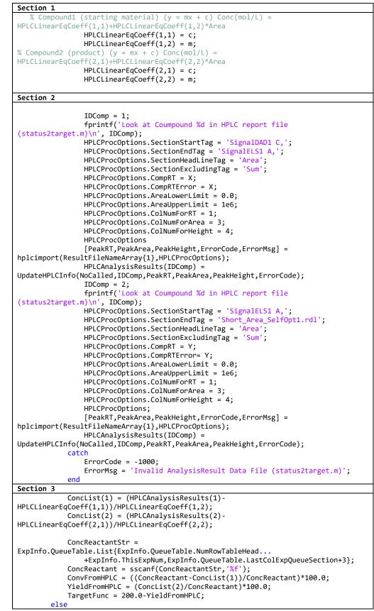
Figure 5.14: Example of status2target.m script file. The file has been reduced to show only the features that are of interest to the operator.
