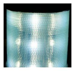
Figure 1.19: Photograph of a microfluidic FEP reactor performing the photo-oxidation of N-methyl-1,2,3,6-tetrahydrophthalimide in acetonitrile using methylene blue as the photosensitiser. The individual substrate and oxygen slugs can be clearly seen in a periodic pattern. Photo taken from Schachtner et al.<sup>147</sup>
