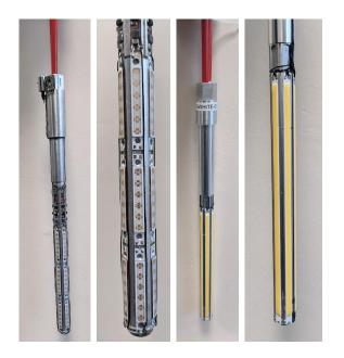
Figure 2.7: Left two images: First-generation PhotoLED with a  $\lambda_{max}$  emission of 424 nm. Right two images: Second-generation PhotoLED, white light emission is generated through the use of blue LED strips coated in yellow phosphor. The two red tubes at the top of the housing are the inlet and outlet for the interior cooling.
