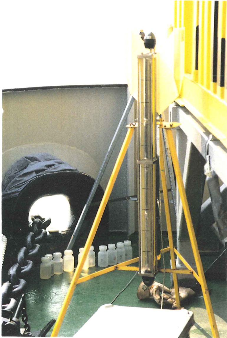
Plate 6 Position of Owen Tube during sub-sampling procedure
