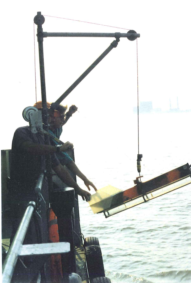
Plate 5 Equipment used for raising and lowering Owen Tube
