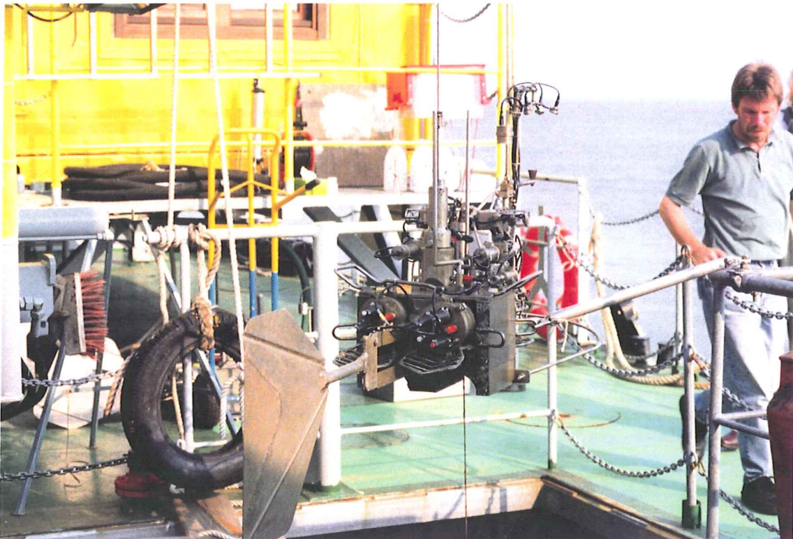
Plate 3 GKSS device for measuring velocity, total suspended matter, salinity and temperature.
